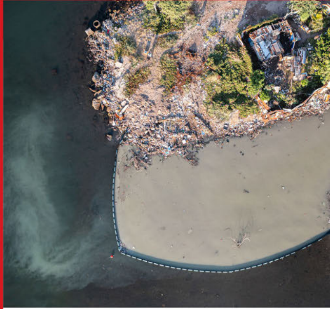
An aerial view of the Interceptor Barrier installed at the mouth of the Rae Town Gully in Kingston. The barrier is part of a pilot project being delivered by the GraceKennedy Foundation (GKF) in partnership with Dutch non-profit environmental organisation The Ocean Cleanup to prevent solid waste entering the Kingston Harbour.
